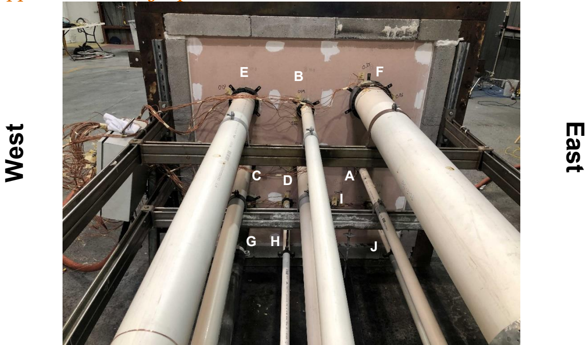
Figure 32 Unexposed face of the specimen before the test
