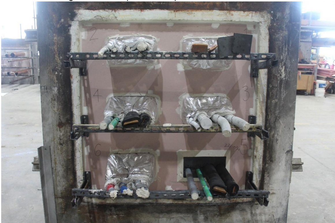
Figure 2 – Exposed face prior to test commencement
